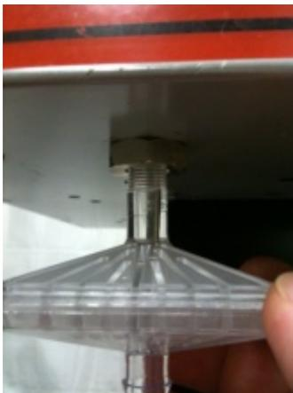
1. Locate the vacuum and filter connection on the left bottom side of the stand body.
